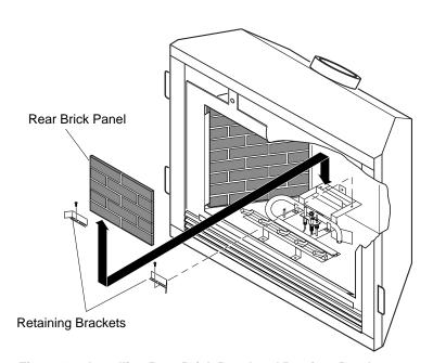
Figure 49 - Installing Rear Brick Panel and Retainer Brackets
